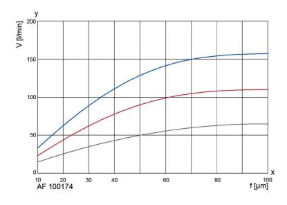
The curves indicate the volume flow through the complete filter system (filter housingh including element) and are referred to a differential pressure of 0.3 bar. Specific process information is essential to guarantee reliable operation of an auto-
