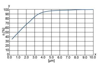
Filtration efficiency: > 98 % at 6  $\mu m$
