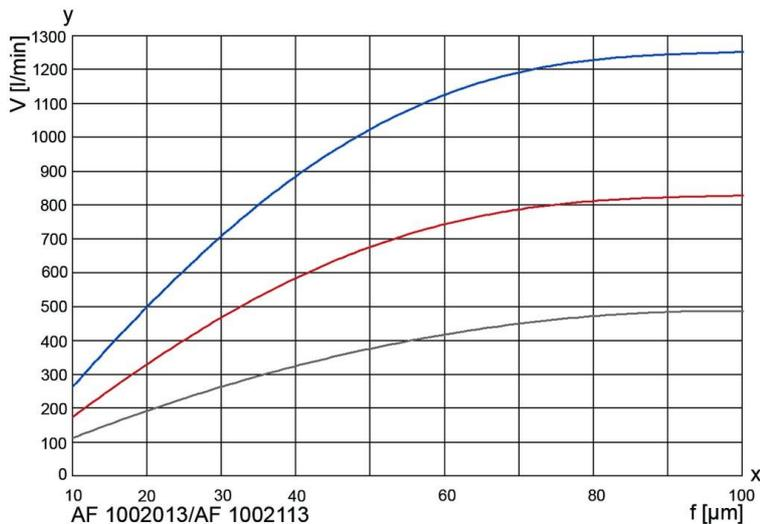
The curves indicate the volume flow through the complete filter system (filter housing including cartridge) and are referred to a differential pressure of 0.3 bar. Specific process information is essential to guarantee reliable operation of an automatic filter.
