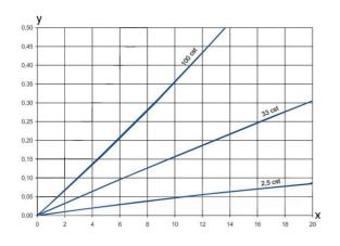
y = differential pressure in bar x = flow rate in l/min
