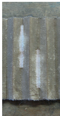
Figure 2: Consequences of pleat-blockage
